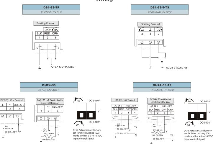
NOTE - To avoid excessive wear or drive time on the motor, use a controller and/or software that provides a time-out function to remove the signal at the end of rotation (stall).
